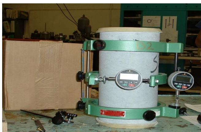
Figure 2: Set-up of cylindrical specimen with Compressometer and Dial gauges for static elasticity test.
